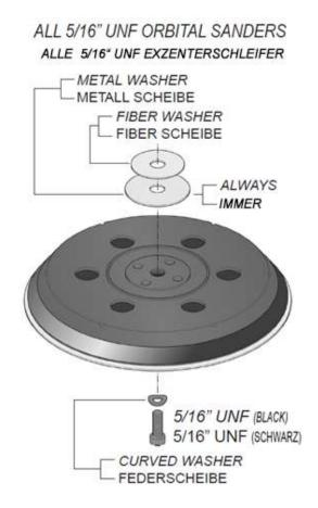
There is no backing pad included in the scope of delivery of the Audurra Random Orbital Sanders. These machines can be used with every established undamaged backing pad. This has no impact on warranty issued and increases flexibility.
